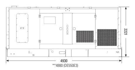
Approximate weight of enclosure package: 5071 kg (11180 lb), \*\*5300 kg (11685 lb) DE550E3. Exact weight is dependent on options. Enclosure weight includes: sound attenuated enclosure, exhaust system, base and generator set.
